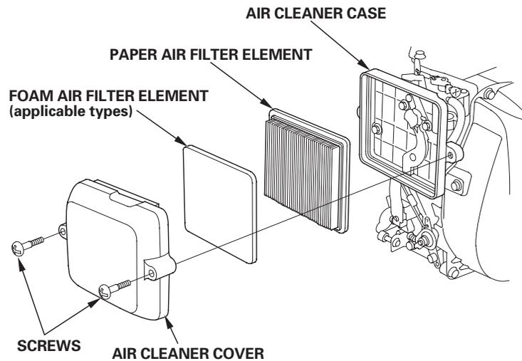
4. Inspect both air filter elements, and replace them if they are damaged. Always replace the paper air filter element at the scheduled interval (see page 6).
