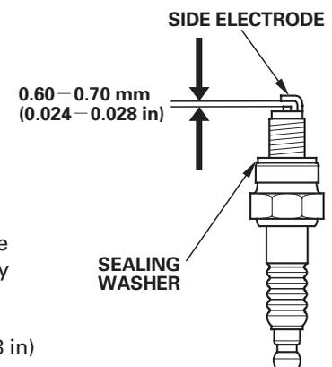
5. Install the spark plug carefully, by hand, to avoid cross-threading.
