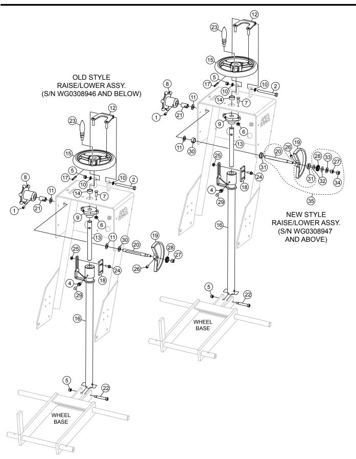
PAGE 12 — SP118 PAVEMENT SAW • PARTS MANUAL — REV. #1 (07/29/10)
