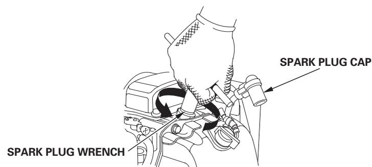
3. Inspect the spark plug. Replace it if damaged or badly fouled, if the sealing washer is in poor condition, or if the electrode is worn.
