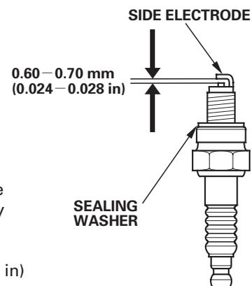
5. Install the spark plug carefully, by hand, to avoid cross-threading.
