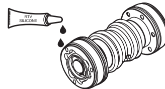
Figure 37. Applying RVT Silicone
