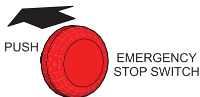
Figure 18. Emergency Stop Switch (Push)
