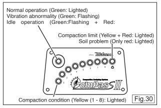
Normal compaction (during compacting) Green LED lights up when the sensor finds that the machine is in normal compaction process. When the revolution goes up, and compaction starts, the yellow LED ① lights up, and as the compaction proceeds, the number of the lighted LEDs increases from ② to ⑧. After the LED light that was calibrated with the measured soil stiffness value lights up, the compaction process completes. (Fig. 31)
