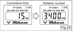
6 After the engine has started, warm up the engine at low speed for 2 to 3 minutes. This is especially important in cold weather.
