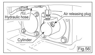
2 After the oil is drained, attach the hydraulic hose again to the cylinder on the vibrator side. With the direction control lever at the forward-most position, fix to the hook with a rope to immobilize. (Fig.56, 57)
