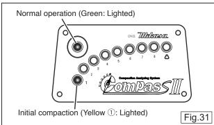
2 Normal compaction (Compaction limit) Compaction limit is reached when all the yellow LEDs from ① to ⑧ have lit up and the red LED lights up. At this point, this machine cannot do any further compaction. If higher soil stiffness value is required, please use a machine of higher level. (Fig. 32)
