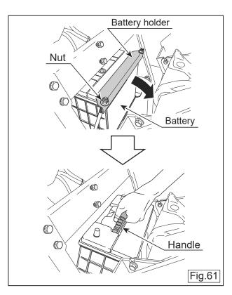
5 For assembly, take the reverse steps described above, but when attaching the battery terminal, start with the red terminal of the plus side. Also, attach securely so that it will not get loosened by vibration.
